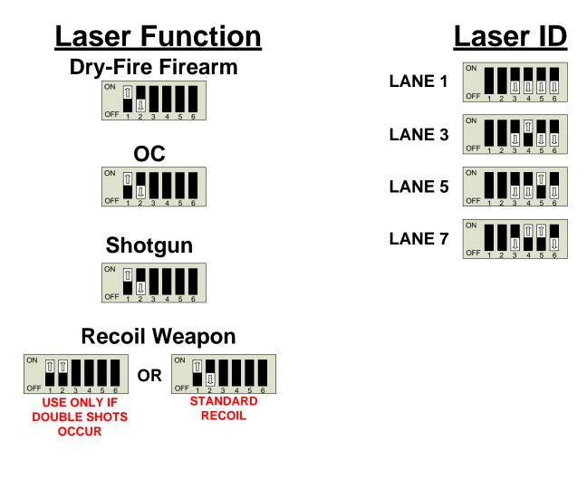
**Switch # 1** determines the "mode" the laser operates in. When off, it provides the traditional 4-lane ID operation. When on, it allows 4x4 and 4x2 operation.
