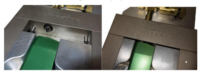
4) If you intend to purge the magazine: Hold the fill handle down and close off the red shutoff valve. When the **red valve** is closed, open the **black shutoff valve** and the contents of the magazine will be discharged through the back of the cradle. Purging will cool the magazine off and allows for the magazine to be filled to a greater capacity. You can purge and fill repeatedly by alternating the black and red valve to fill and then dump the contents of the magazine.
