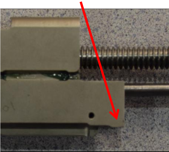
Semi-Automatic Recoil Bolt Assembly without Flange
