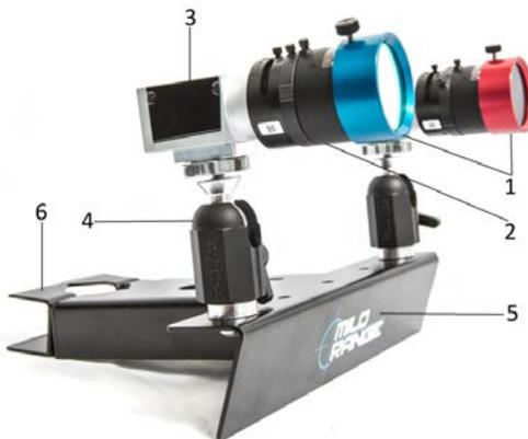
**Figure 11 – Camera Tree with Cameras attached**
