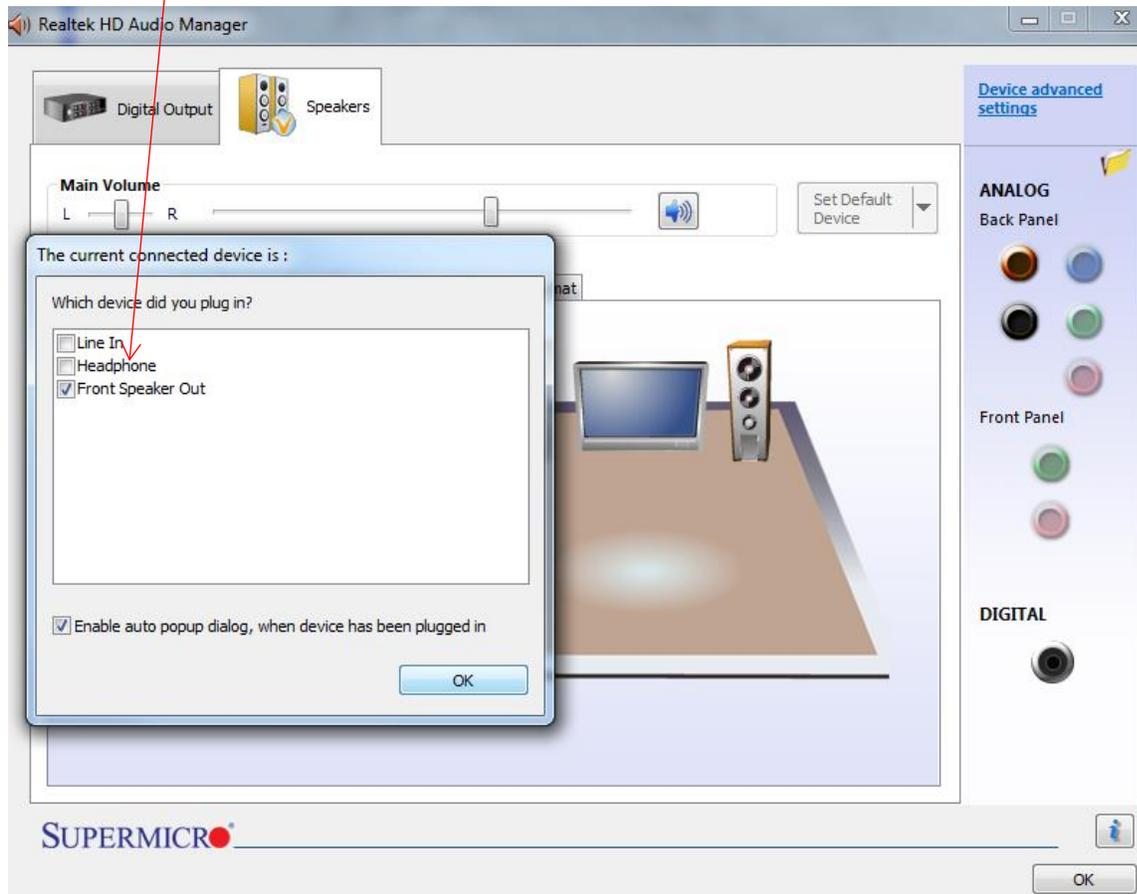
After plugging in the green analog cable, the dialog box below will appear. Be sure to check the box Rear Speaker Out. Then click ok.
