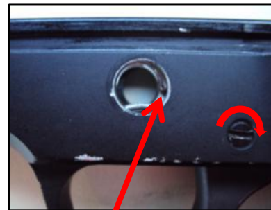
Locking Insert Blocking Takedown Lever Hole Remove Recoil Locking Insert & Rotate Trigger Pivot 180 degrees
