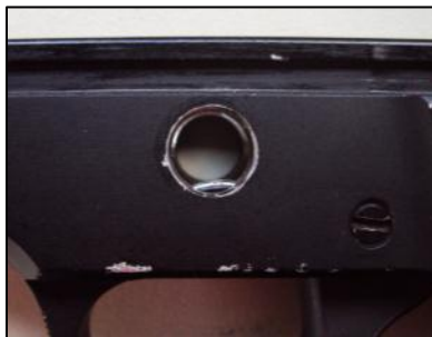
Locking Insert Fully Seated Correct Trigger Pivot Position Takedown Lever Hole is Clear
