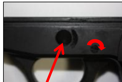
Locking Insert Blocking Takedown Lever Hole Remove Recoil Locking Insert & Rotate Trigger Pivot 180 degrees
