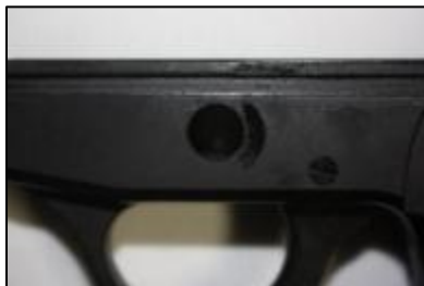
Locking Insert Fully Seated Correct Trigger Pivot Position Takedown Lever Hole is Clear
