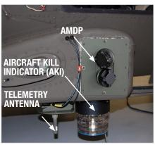
AMDPs are installed and connected to the aircraft Laser Warning
