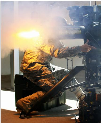
ITAS-TESS features a boresighting capability, aided target tracking, embedded training, and built-in test (BIT). The ITAS TESS system can be used in a fully instrumented mode telemetering all data in real time, or a Laser only mode for crew level, laser based training. Training event data is passively collected and transmitted to a Mobile Command and Control (MCC) display and monitoring system for playback and After Action Review (AAR).
