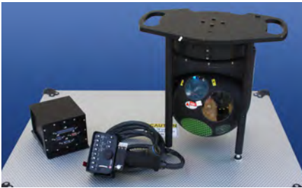
Articulating Sensor Package (ASP) with FlashWESS Laser Transmitter (FLT), Weapons Processor & Hand Controller
