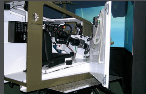
Common Driver Trainer High-Fidelity Manufactured Cab
