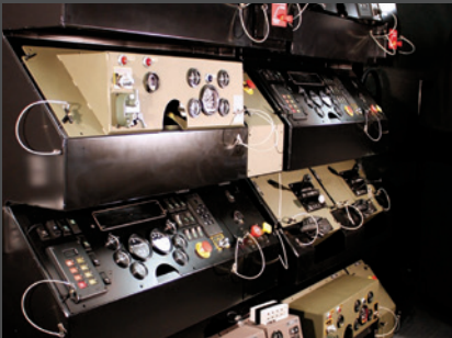
Fabricated ODS Cab with Interchangeable dash panels
