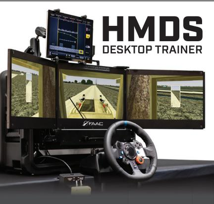
The HMDS Desktop Trainer uses the same software and touch screen interface as found on the VCTS and operational HMDS, therefore, providing a seamless training capability. By design, the HMDS DT is easy to operate by unit personnel. Upon fielding, the BEB Route Clearance platoons will now have the ability to train VMMO operators on proper HMDS employment, operation, and detection of explosive hazards.
