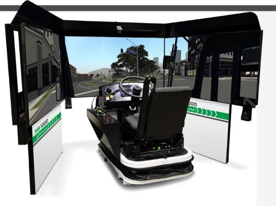
The MB 1000, with its more than 225-degree field-of-view capability, realistic dash controls, and optional motion system, is a testament to the innovative solution FAAC provides to the transit industry.
